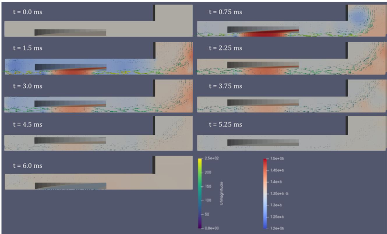
**Figure 5: Plate position, pressure (red/blue) and gas velocity vectors (green/yellow) as a function of time for one cycle of the valve. The first impact occurs after 1 ms, while second impact occurs after 2.4 ms. After impact, a region of lower pressure is seen above the valve, contributing to the damping phenomenon.**
