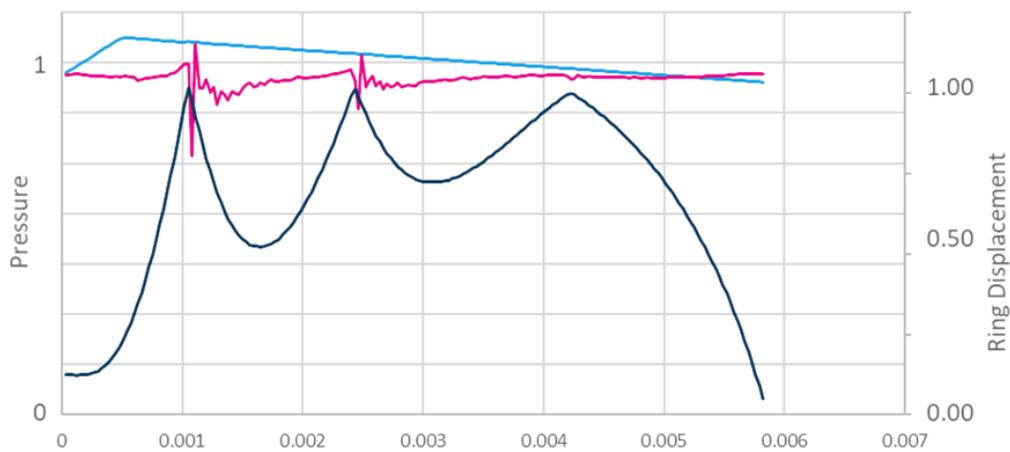
**Figure 6: The normalized pressure on bottom side (light blue) and top side (purple) of the ring plate, as well as the normalized valve lift (dark blue).**
