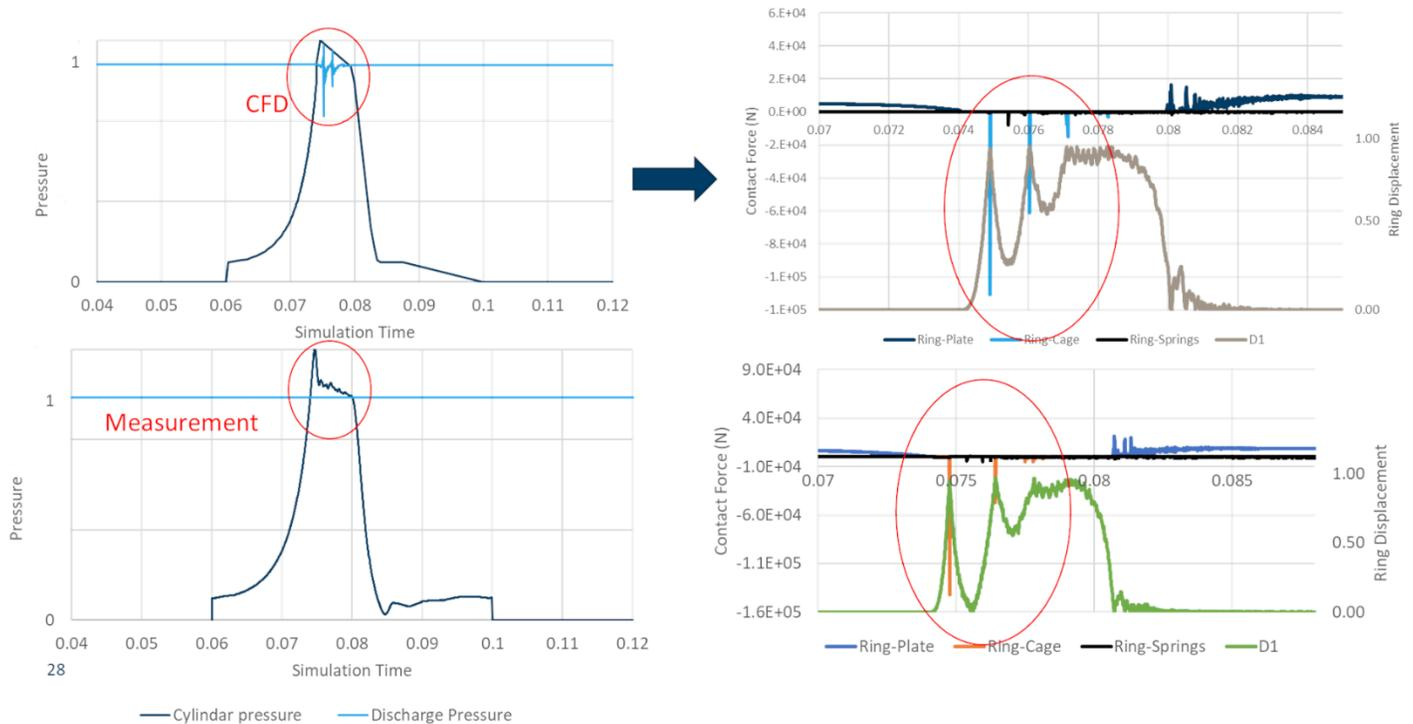
**Figure 7: Using pressure from CFD in FEM (top), vs. using pressure from experimental measurements (bottom). The pressure cannot be measured at the top and bottom of the valve plate but is taken further away.**
