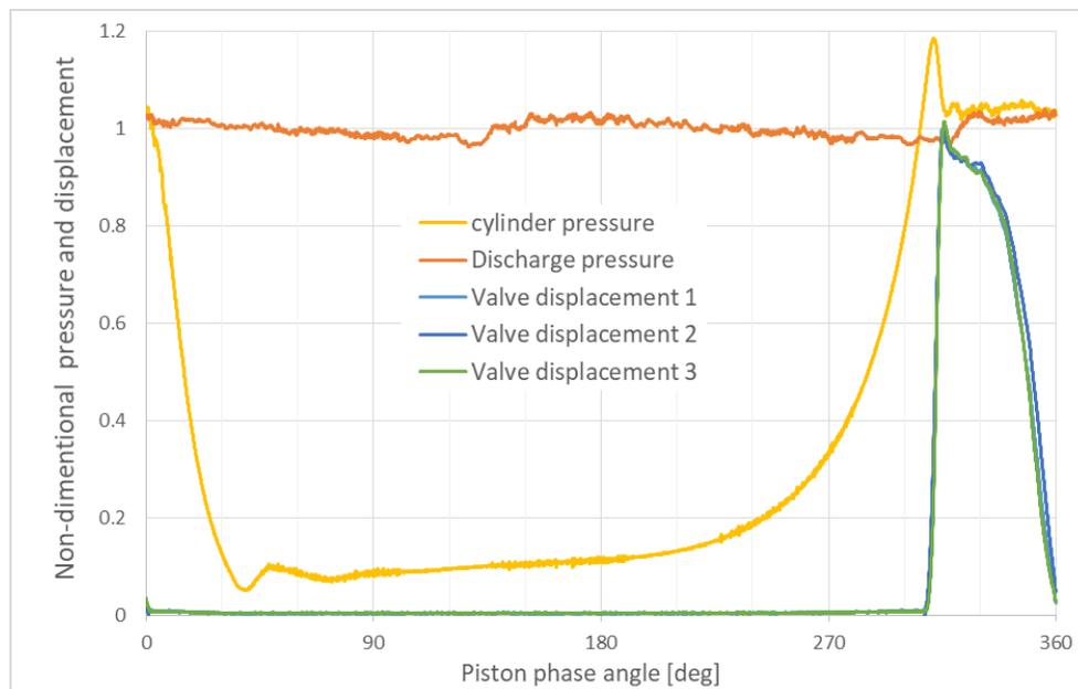
**Figure 4: Measured values of cylinder pressure, discharge pressure and valve displacement at working conditions.**
