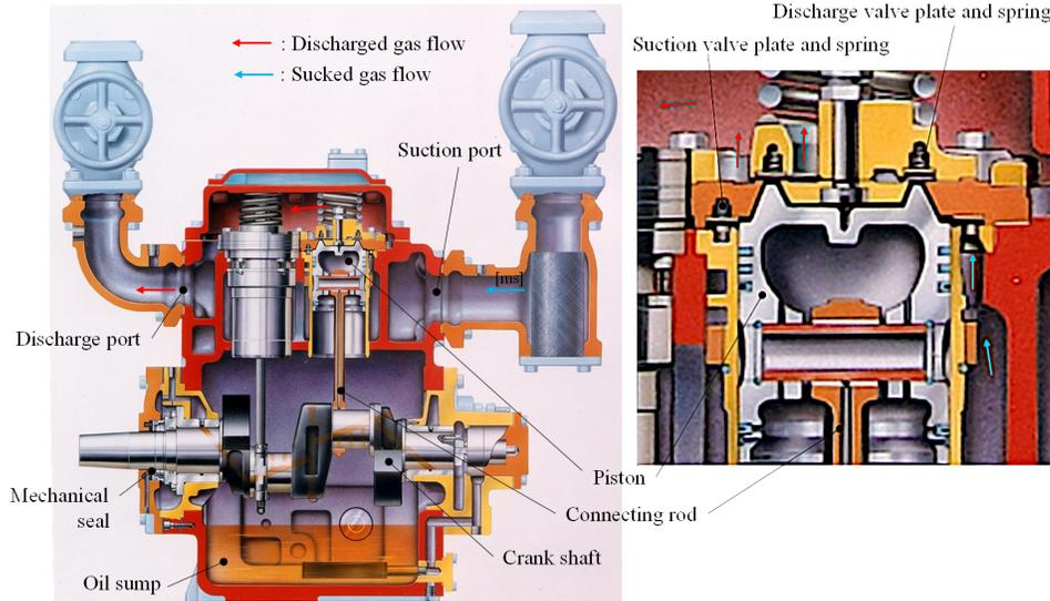
Figure 1: Illustration of the piston compressor and valves.
