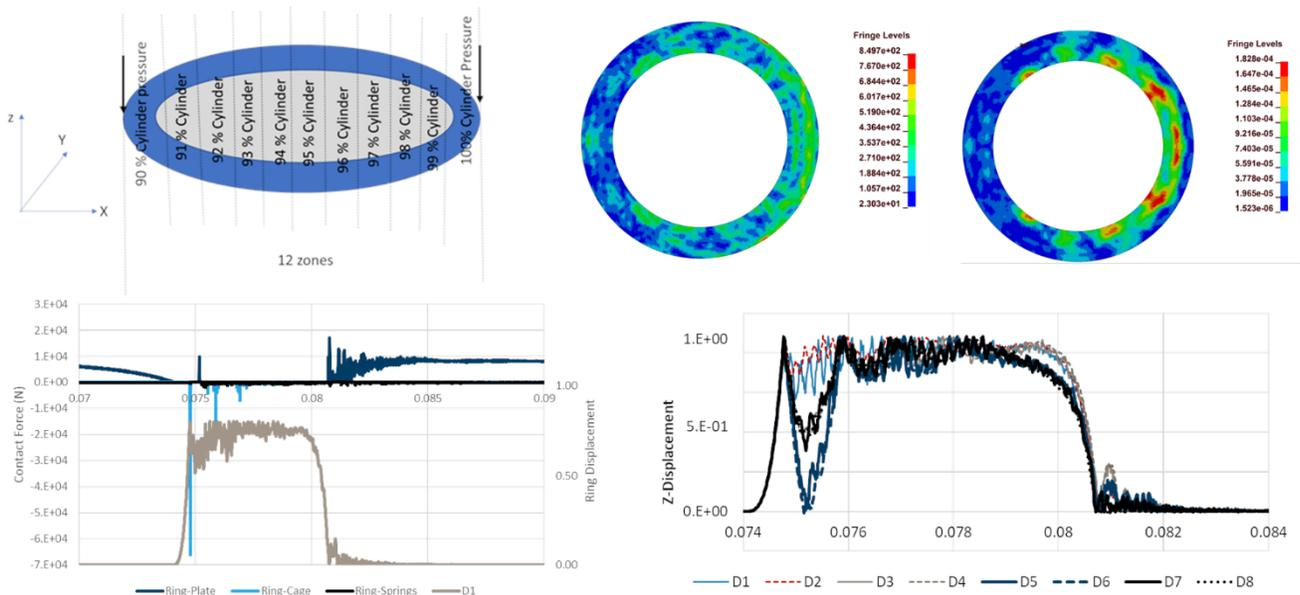
**Figure 6: Response to asymmetric pressure distribution on the valve plate.**
