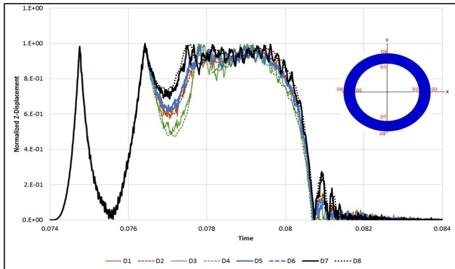
**Figure 5: Displacement curves of 8 nodes distributed on the surface of the ring as illustrated in the inset figure.**
