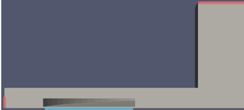
**Figure 2: Cross-section of the valve cage geometry used in the CFD. The inlet from cylinder is shown in blue, and the outlets are shown in red.**
