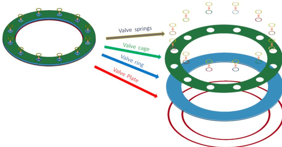
**Figure 3: Illustration of the geometry and setup of FE model.**
