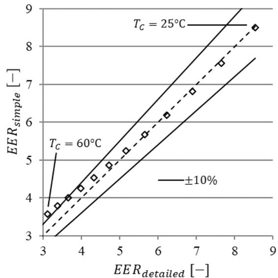
**Figure 6: Deviation of the simple and the detailed model at varying condensation temperatures**
