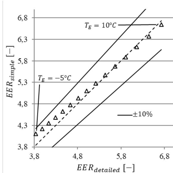
**Figure 4: Deviation of the simple and the detailed model at varying evaporation temperatures**
