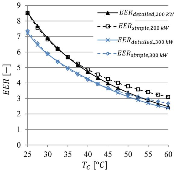
**Figure 5: Comparison of EER values obtained from detailed and simple model at varying condensation temperatures**
